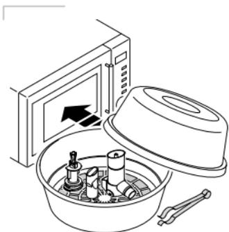
⇒ Place the components in the disinfector with enough space between them. If possible, place the parts in the appliance so that the steam created by the microwave action can flow through the parts to the greatest effect.
